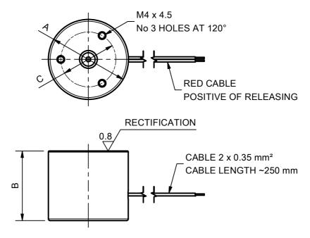
N.B. THE SURFACE RECTIFIED BY MEANS OF NO GALVANIZING, MUST BE KEPT LUBRICATED SO AS TO AVOID OXIDE FORMATIONS
